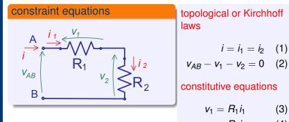
$$v_2 = R_2 i_2 \qquad (4)$$
